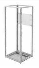
Partial Mounting Plates are conductive, unpainted 2,5 mm galvanized steel and have flanges on four sides. Panels can be positioned vertically in 25 mm increments and also can be positioned at any depth in 25 mm increments using the optional depth grid straps (order separately). All necessary mounting hardware is included.
