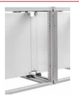
Provides a continuous panel surface in multiple-bay enclosures. The joining mounting plate is inserted between mounting plate of equal height. It can be installed from front or rear. Holes for grounding and mounting hardware are provided. Conductive mounting plates are unpainted galvanized steel.
